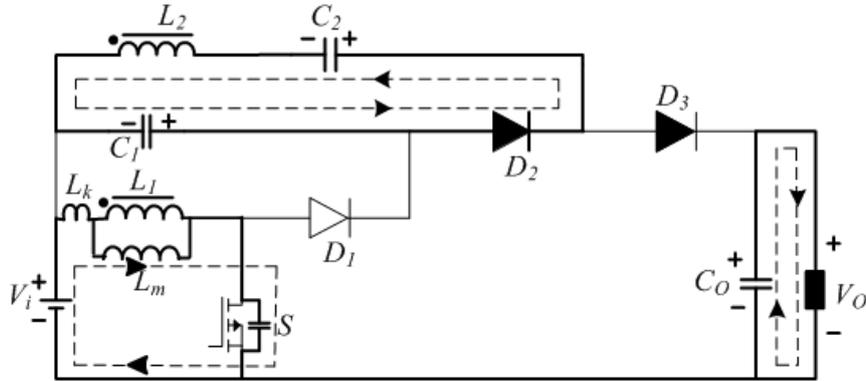
$$i_{Lk}(t) = \frac{V_{C1}}{L_m + L_k}(t - t_2) + i_{Lm}(t_2) \quad (3)$$
